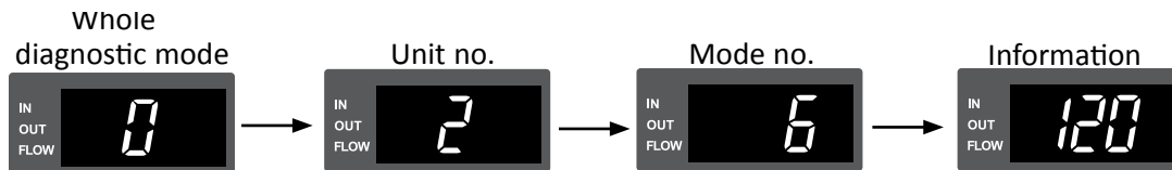
Figure 40. This example shows the steps for displaying the outlet temperature for unit 2 in a linked system.
